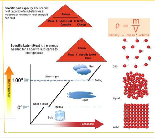
Specific latent heat is the energy taken to make 1Kg of substance change state.
